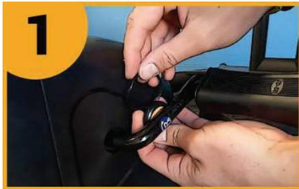
**1 - Attaching the sensor to the pedal crank:** Start by attaching the CycloSense sensor to your bike's pedal crank using the provided Velcro strap. Ensure that the sensor is securely fastened to ensure accurate measurements.
